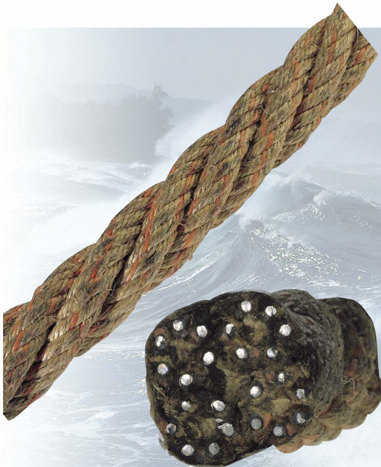
REF. TR - 015 DIAMETER 53 MM., 4x6 - MBL = 27.5 TONS.
